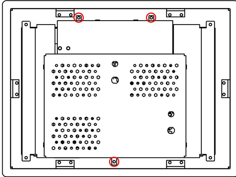
2. Carefully remove the metal cover by pulling it upwards.
