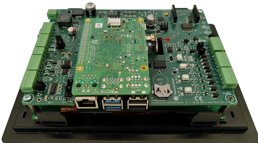
4. Finally, remove the Raspberry Pi by pulling it upwards. Keep in mind that it is fixed to the main PCB by 4 plastic supports and be careful not to bend any pin of the Raspberry Pi GPIO header.
